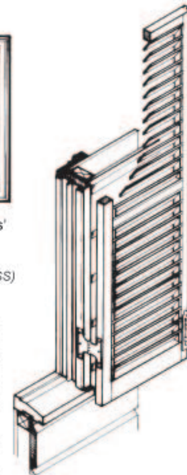
"Cut-away" view of window shutters
