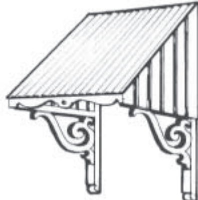
Woodworkers' Sweep Skillion Shown with fretwork fascia option Overhang 565 mm Height 1300 mm WH 4
